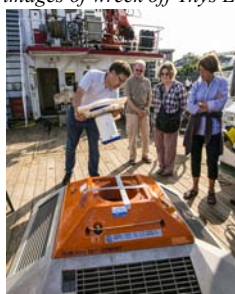
Monitor for measuring temperature & salinity at various depths
