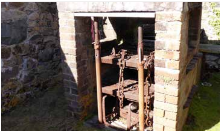
The unique chain cleaning furnace
